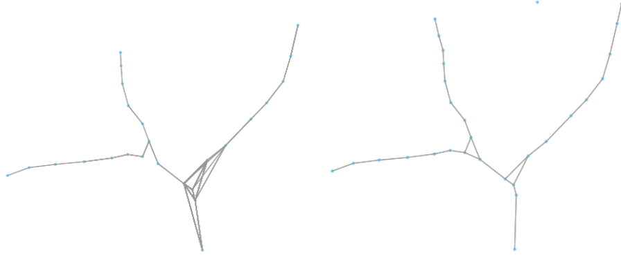
Figure 1: From left to right: Helsinki area produced by the failed, geometry based simplification; Helsinki area produced by the successful, image based simplification
